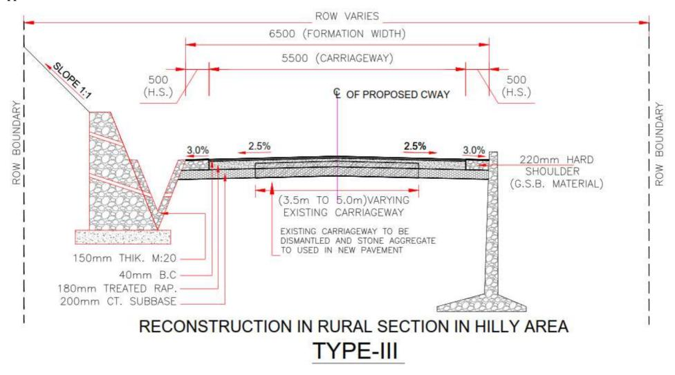
\* Retaining wall and Breast wall shown in TCS III drawing is typical. Location of these components should be applied as per site condition.
